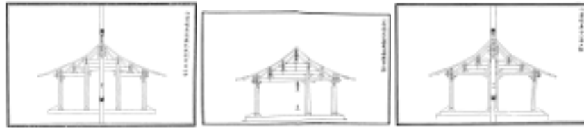
Figure 1. Drawings and written descriptions of building sections in the Yingzao fashi . Shown here are the three sections of six rafters' depth (Liang 1983, 319–320).
